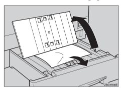
While opening the guide in step **2**, open the two guides as shown in the illustration.
